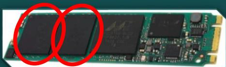
**DRAM:** Temporary storage - faster than NAND - buffer between controller and NAND to increase speed.
